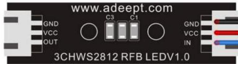
WS2812 LED is a very common module on our robot products. There are three WS2812 lights on each module. Please pay attention to the signal line when connecting. The signal line needs to be connected to WS2812 after being led out from the Raspberry Pi. The "IN" end of the LED light module.
