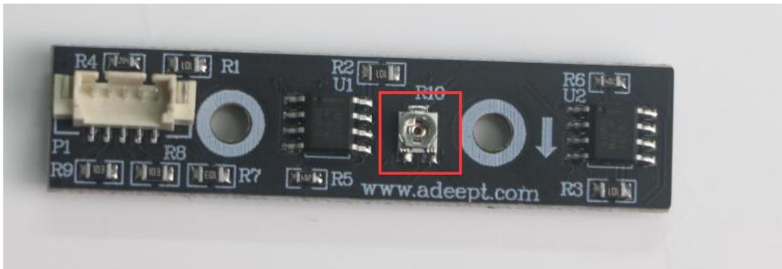
8. After debugging, you can test LF2 and LF3. When LF2 or LF3 is placed above the black line, D2 and D3 corresponding to the WS2812 LED will also light up in blue.
